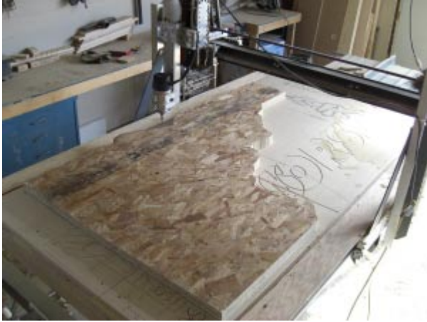
Rough Machining the map of Idaho
