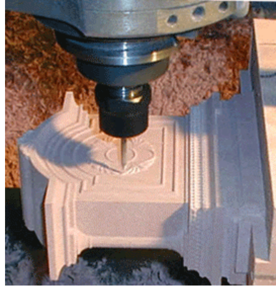
Machining of the front and back of a mantle piece clock on a Fadal vertical machining center
