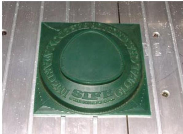
**Figure 1** – This image shows an early wax prototype of the award created by Professor Hollern and Pamela Argentieri, and machined with VisualMill.
