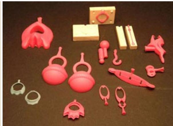
**Figure 6** – Detail of design from student Kyle Bradford that was machine with VisualMill.
