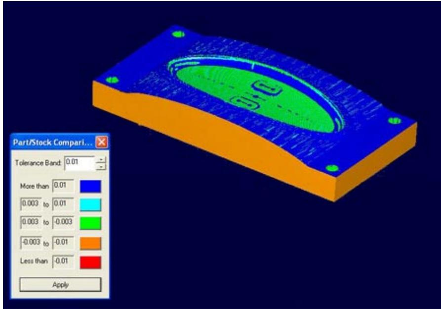
**Figure 5** – The Jacuzzi part was built in SolidWorks and it takes 90 seconds to regenerate, due to its complex internal shapes. However, it imported without a hitch into VisualMill, which also had no problem creating a toolpath. The final part can be seen in figure 1.
