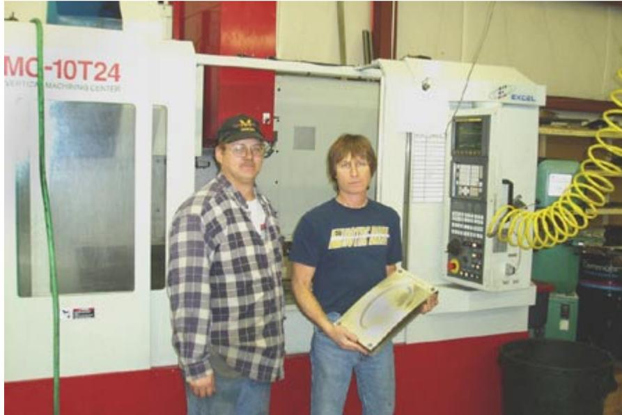
**Figure 1** - Mike Eaton and Chris Fletcher of Jessco Manufacturing Inc. stand in front of one of their two CNC machines. Mike Eaton is holding a cavity of a mold for a Jacuzzi component, which was just machined with tools controlled by VisualMill.
