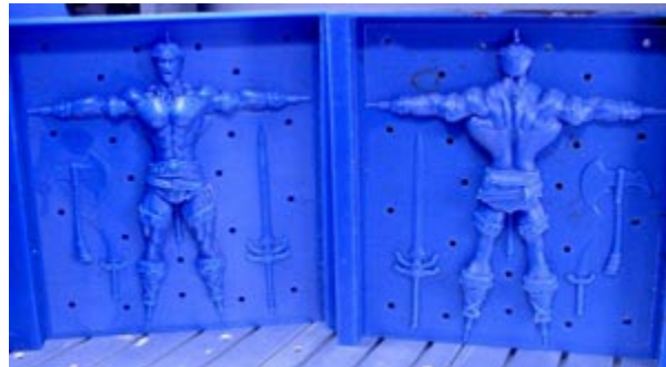
Figure 2: A toy figure Barschdorf created, machined and cast with the help of VisualMill.
