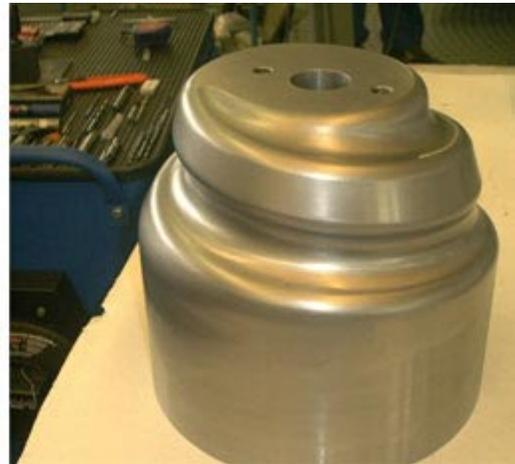
**Machined parts programmed in VisualMill**
