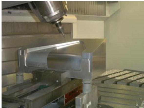
**5th Axis Machining In-Progress**
