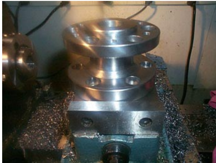
Fig 5 – Part machined in VisualMill.
