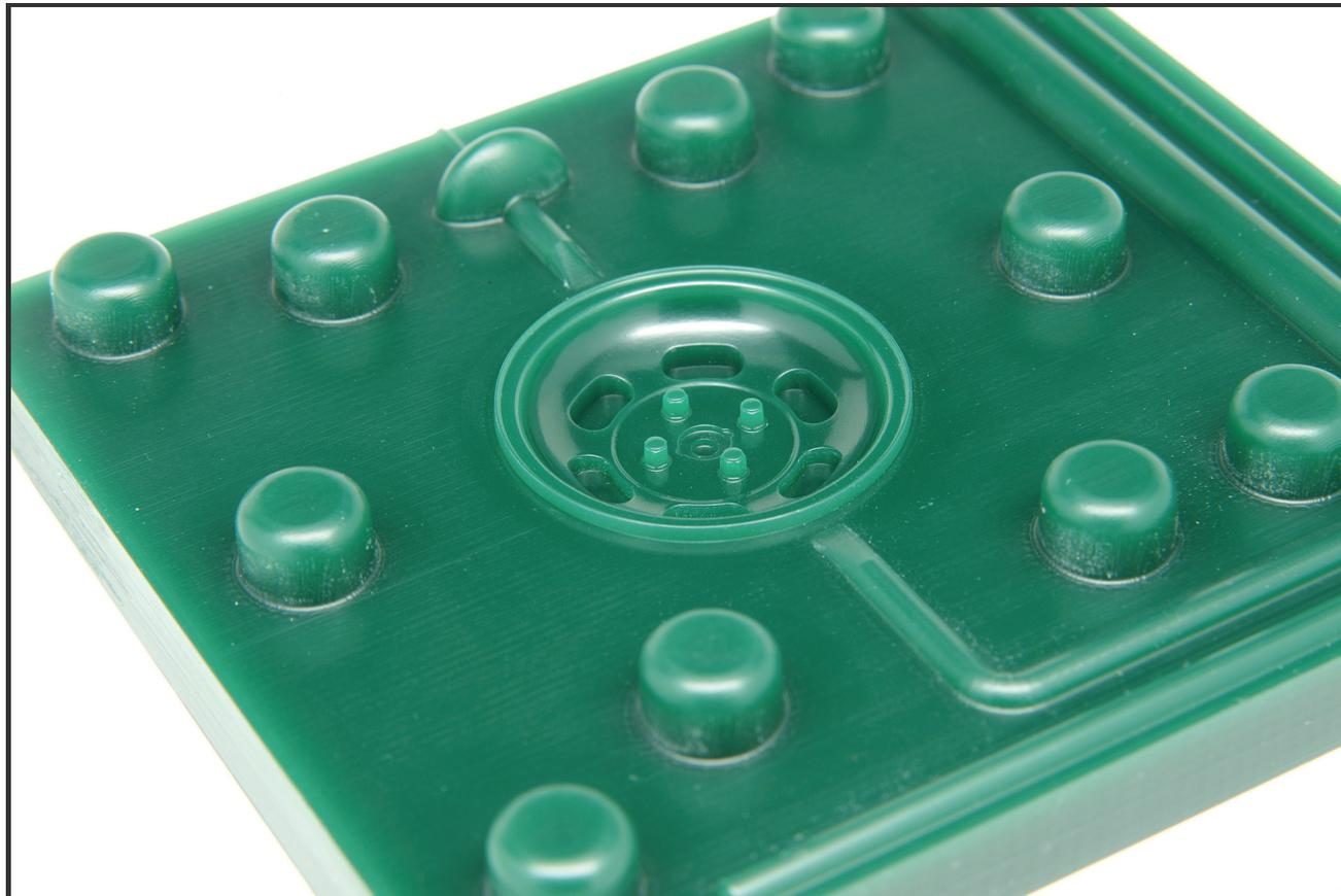
The prototype positive wax top mold cavity of the Riverview Hobbies RVH121001 Slotted Mag Wheel Kit
