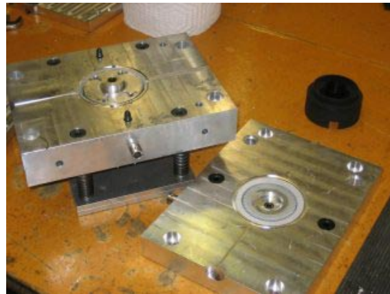
Example of a typical plastic injection part and mold that Larry makes
