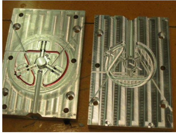
Machining of Aluminum molds for plastic injection prototypes
