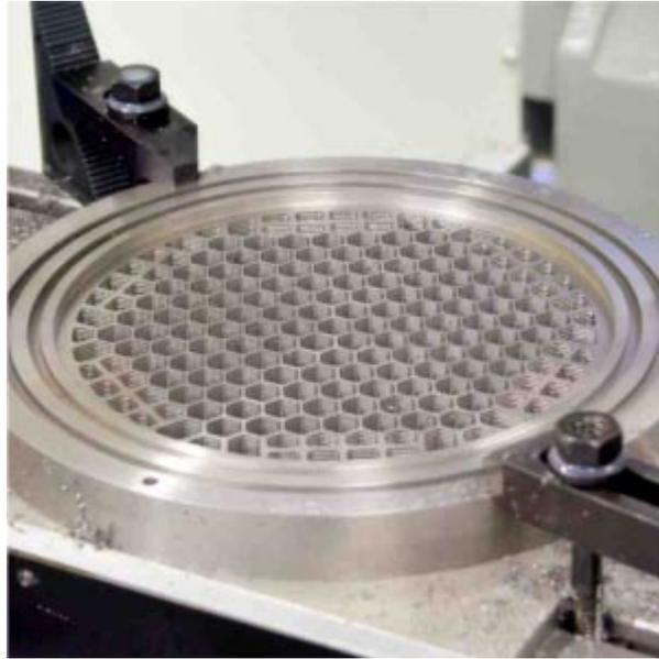
Stainless Steel Plate - 12" diameter x 1.25" thick. Approximately 190 holes with stress optimized webs - Approximately 2-hours programming (and test cuts), 8-hours machining time. Outstanding Results!
