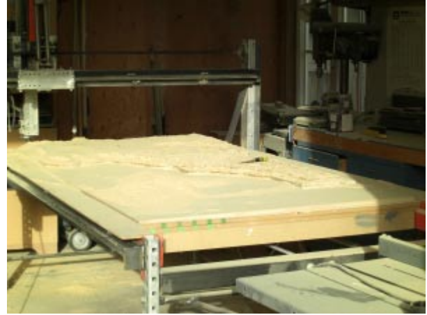
Map after Finish Machining
