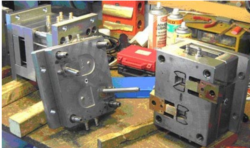
Plastic injection molds machined and produced using VisualMill
